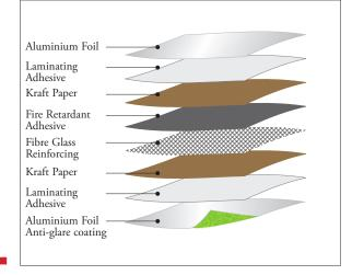
has a green antiglare which is installed to the outside of the building to reduce reflection to acceptable levels. Due to its unique construction, Thermofoil Medium Duty sarking has a medium water vapour transmission rate making it suitable for light weight wall cladding applications that are batten fixed, battens thereby providing the required air space of 20mm in between cladding and the foil.
